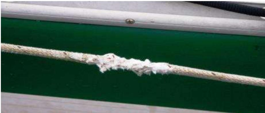
Lines may begin to wear in the middle due to the snapping action when the boat is pitching.
